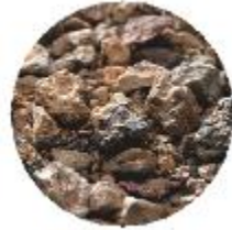
AGGNEO Recycled aggregates from construction demolition waste
